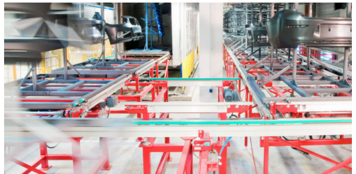
Skid conveyor with space-saving lateral travel for changing direction.
