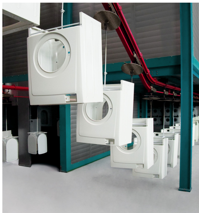
Climbing circular conveyor with oven and A lock.
