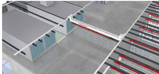
Paint shop for trailer – transfer bridge with carrier set.
